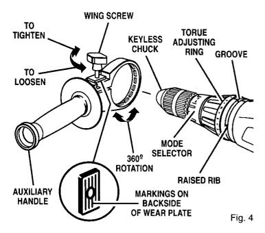
To prevent possible loss of control, auxiliary handle should be checked periodically for tightness. **Do not operate hammer drill with auxiliary handle loose.**
